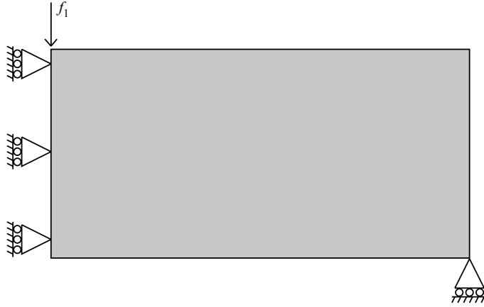
Figure 3.1: Design domain used for all the examples in Chapter 3. Dimensions are 60 units in the horizontal direction and 30 units in the vertical direction. The loads and boundary conditions in the design domain correspond to half the MBB-beam.
